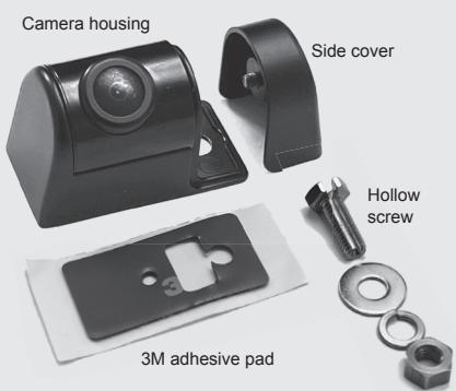
Insert the cable into the groove from the hollow thread screw. Route the cable with the hollow thread screw into the round hole in the camera base. Drill a mounting / cable cable feed-through hole with a diameter of 6 mm. Fix the cam via hollow threaded screw with washer, spring washer and M6 lock nut.
