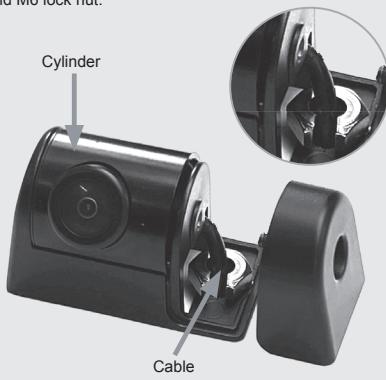
Alternatively, the camera can be fixed with the 3M adhesive pad or the self-tapping screw. The cable must always be routed though the round hole in the camera base to provide for full adjustment range of the sensor cylinder. Loosely screw on the housing cover and align the camera. Tighten the locking screw well.
