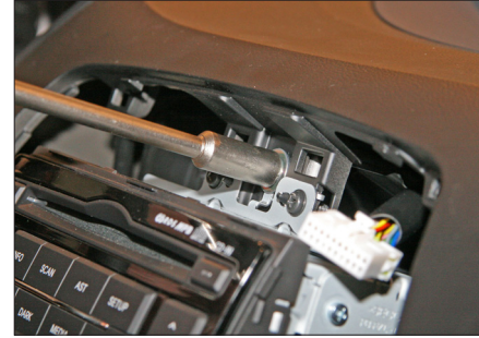
5. Remove screw on top of OEM head unit
