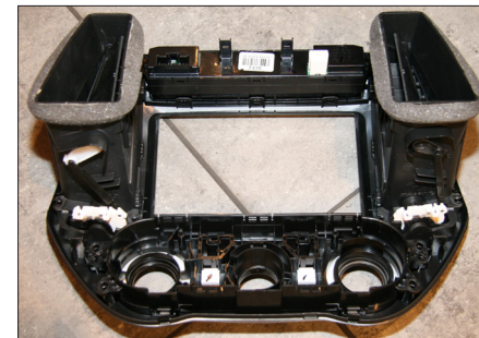
8. Mount OEM air vents to new facia plate Mount hazard light switch to new facia plate
