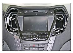
3. Remove 4 screws at left and right side of OEM head unit (see arrows)
