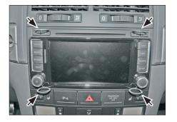
Put four radio release keys in the appropriate slots of the OEM head unit.
