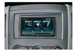
5. Place the facia plate on the dashboard. Fix it with the four original screws.
