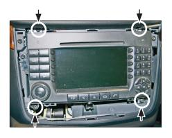
Remove the four screws at the top and bottom of OEM head unit.
