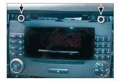
Remove the two screws at the top of the OEM head unit.
