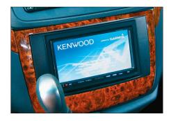
4. Place the facia plate on the dashboard. Fix it with the four original screws.
