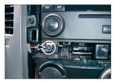
Remove the two screws below the OEM head unit at each side.
