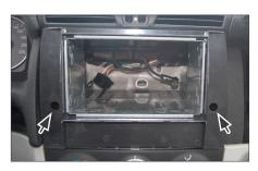
4. Push the metal frame into the mounting frame.
