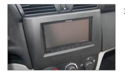
3. Connect all required circuit points and push the double DIN head unit in the metal frame until it snaps in.
