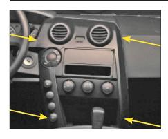
1. Remove the panel under the climate control panel.
