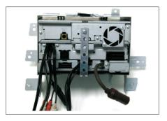
6. Tighten the headunit onto the metal band. Various positions are possible.
