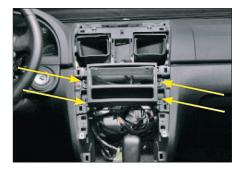
3. Remove the original bracket. This is tighten by screws.
