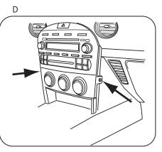
Pull radio/climate control panel out, disconnect plugs and remove. (Figure E)
