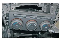
6. Remove the air condition control unit
