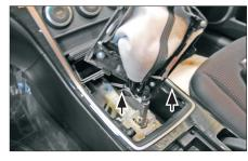
2. Remove the gear shift cover
