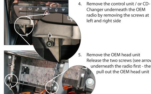
radio by removing the screws at left and right side
