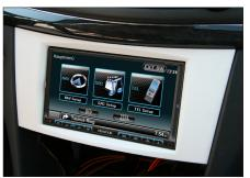
Push the facia plate onto the mounting bracket
