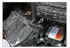
Open the ash tray and remove the complete ash tray unit
