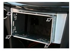
Push the metal frame into the mounting bracket
