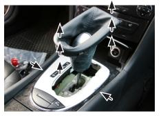
Pull up the gear shift cover Unclip the gear shift panel and remove it
