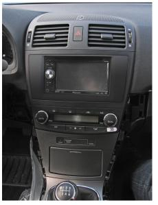
7. Install Double DIN head unit (using OEM mounting frames)
