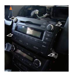
6. Remove 4 screws securing
