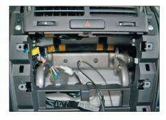
3. Remove the OEM head unit (which is still mounted to the metal cage)
