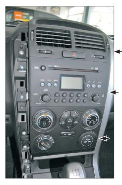
Remove the side panels at the left and right side of the dashboard
