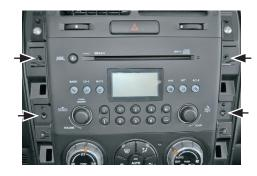
2. Remove the four screws beside the OEM head unit.
