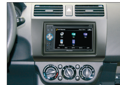
Connect alle required circuit points and wires. Push the double DIN head unit until it snaps in. Place plastic radio trim. Place back all panels in reverse order.
