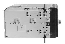
4. Mount the metal brackets with the double DIN head unit
