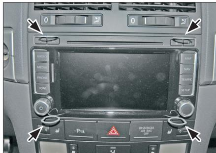
2. Put four radio release keys in the appropriate slots of the OEM head unit.
