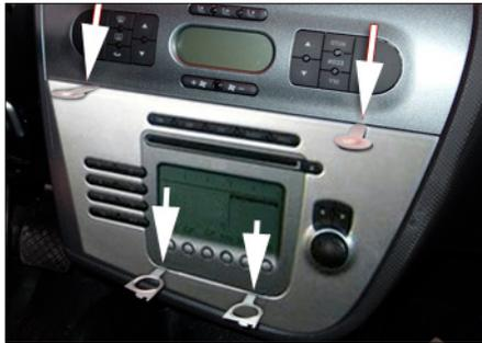
3. Insert 4 radio release keys into slots on the top and bottom of the radio (see arrows)
