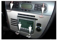
Insert 4 radio release keys into slots on the top and bottom of the radio (see arrows) Mount the metal brackets to the double DIN head unit.
