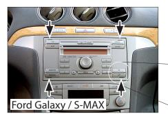
Insert Ford radio release keys in the holes of the OEM head unit.
