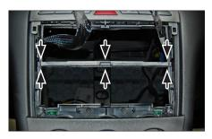
Remove middle bar to clear space for the Double DIN head unit.
