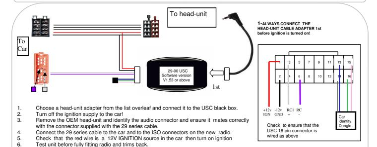
If Problems: Check that correct adapter has been used and links are in the correct place. Always disconnect from the power supply if you change the head-unit adapter lead. Check that Red wire is 12V ignition and not Permanent power. Check that head-unit is earthed and black wire is earth. Check all connections are the same as the wiring diagram shown here
