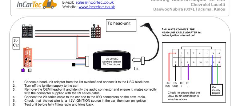
If Problems: Check that correct adapter has been used and links are in the correct place. Always disconnect from the power supply if you change the head-unit adapter lead. Check that Red wire is 12V ignition and not Permanent power. Check that head-unit is earthed and black wire is earth. Check all connections are the same as the wiring diagram shown here
