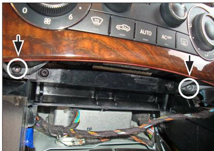
3. Remove the two Torx (TX20) screws underneath the air condition control unit.
