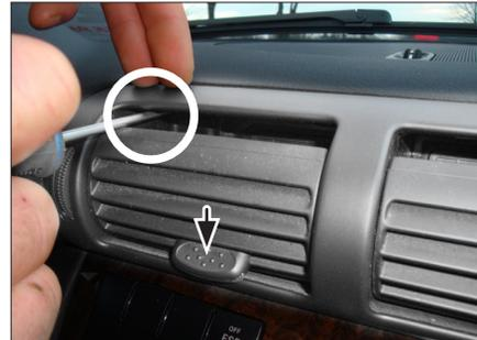
7. Pull down the air vent and unclip the whole unit at both sides carefully with a screw driver.
