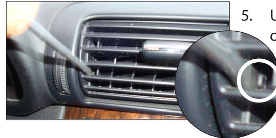
5. Unclip the air vent unit carefully on both sides with a screw driver.
