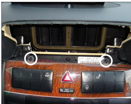
8. Remove the two Torx screws, located over the switch panel. Remove the switch panel.
