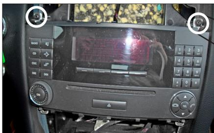
9. Remove the two Torx screws, located over the OEM head unit.
