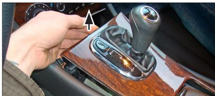
2. Remove panel by lifting it up. Remove ash tray.
