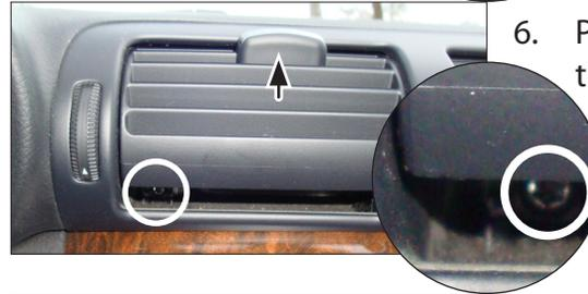
6. Pull up the air vent and remove the 2 screws (left and right) which become visible.
