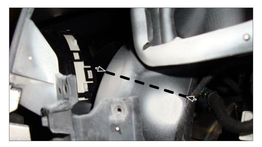
3. Cut here air vents (see dashed line) Insulate holes with duct tape
