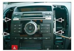
2. Remove screws of OEM head unit
