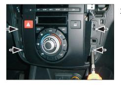
3. Remove screws of control unit (be low OEM head unit)
