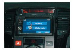
5. Attach brackets to Double DIN head unit. Connect all required circuit points. Fix Double DIN double DIN head unit at dashboard. Place facia plate until it snaps in. Reinstall everything in reverse order to finish installation
