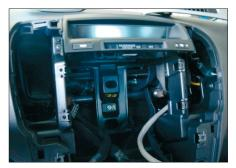
4. Remove OEM head unit and cotrol unit
