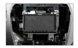
6. Push double DIN head unit into metal frame until it snaps in
