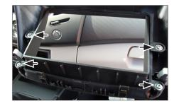
Mount facia plate to OEM-Panel (with original screws)
