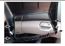
Remove 4 screws to disassemble **OEM-Case from OEM-Panel**
