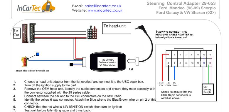
If Problems: Check that correct adapter has been used and links are in the correct place. Always disconnect from the power supply if you change the head-unit adapter lead. Check that Red wire is 12V ignition and not Permanent power. Check that head-unit is earthed and black wire is earth. Check all connections are the same as the wiring diagram shown here
