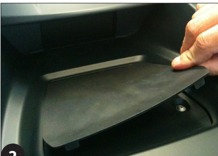
4. Unclip cover of center console
