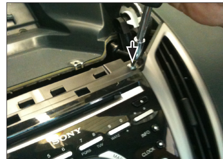
12. Remove screws on top of OEM head unit (left and right)
