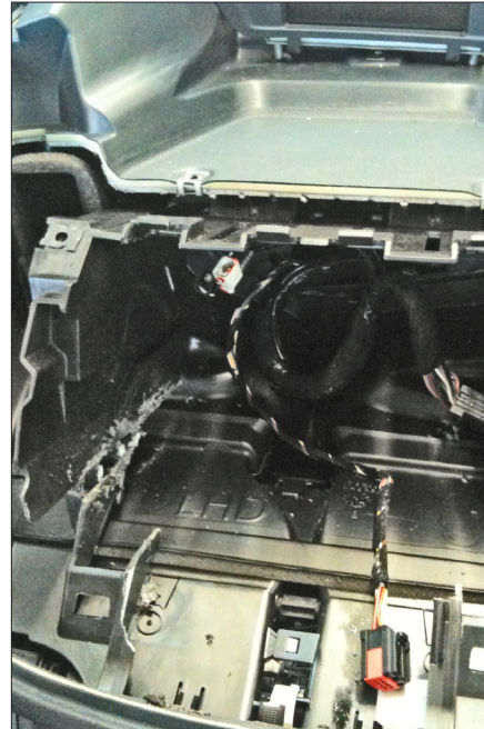
17. Dashboard after plastic cut out
