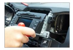
6. Remove screws of OEM head unit
