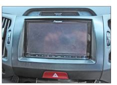
11. Remove hazard light switch (1) from OEM head unit - attach it to double DIN facia plate
