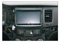
Mount OEM panel to facia plate in case of inaccurate mounting position: cut upper part of OEM panel holder holes (see arrows) to a flat hole in order to get more flexibility for adjustment
