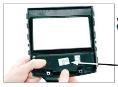
10. Remove OEM panel holding harzard light switch and clock.
