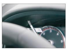
4. Remove 2 screws beneath tachometer unit cover left and right side
