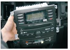
8. Remove screws of OEM-head unit. Remove OEM head unit by pulling it towards your direction
