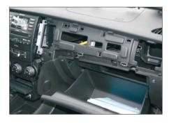
7. Remove whole panel with integrated air vents
