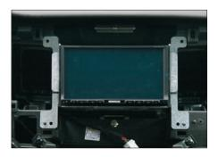
Attach metal mounting brackets to Double-DIN navigation
