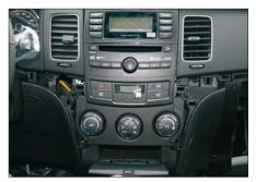
Unclip and remove silver panels at left and right side carefully
