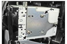
8. Remove 2 screws (see arrows) Remove OEM head unit
