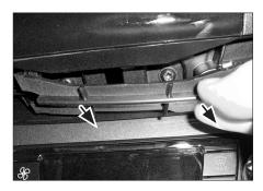
2. Unclip panel under OEM radio
