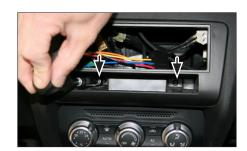
Fix facia plate with 2 OEM screws 6. (removed in step 3)
