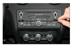
Use special radio release keys to 2. remove head unit (see arrows)
