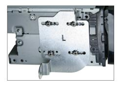
Mount brackets to double DIN Navigation as shown in sample photo
