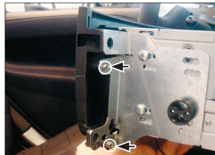
5. Push facia plate over double DIN head unit. Fix facia plate with 2 self-tapping convex fillister head screws (see arrows) at each side
