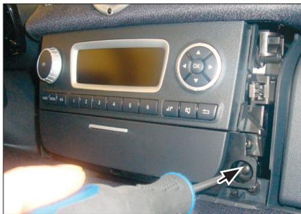
3. Remove screws of tray below OEM head unit (see arrows)
