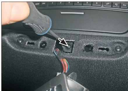
2. Remove screw under hazard light switch (see arrow)
