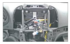
Unclip the center panel and remove it
