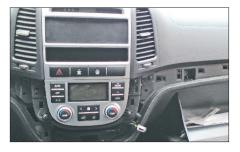
Remove the screws, holding the center panel
