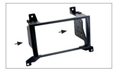
4. Attach the mounting brackets to the facia plate
