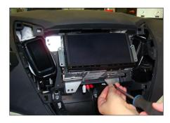
Mount mounting frames to double DIN head unit
