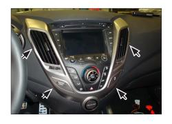
Unclip OEM panel with air vents (see arrows)
