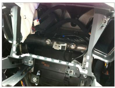
6. cut away here (see lines) to clear space for double DIN head unit
