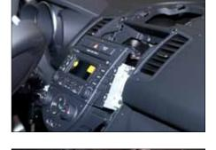
Dash board with removed head unit
