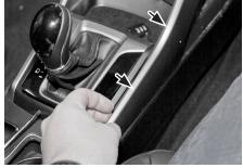
OEM side panels need to be removed. Start at this position (see arrows)
