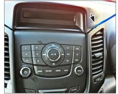
Remove side panelsRemove screws left and right
