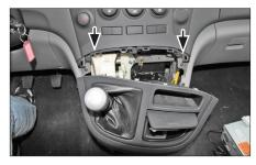
2. Unclip the gear lever box
