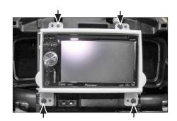
5. Place the Pioneer Navigation with the facia plate at he dash boardConnect all required circuit points
