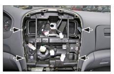
Unclip the front panel and remove it
