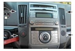
Unclip the air vents on the left and right side of the OEM head unit with a plastic wedge and remove them.
