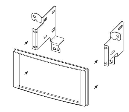
4. Slide double DIN head unit into the brackets/facia plate and secure to the assembly with screws
