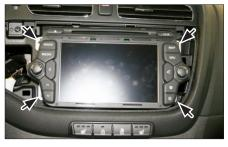
2. Remove screws of OEM head unit
