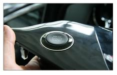
3a. Mount "Engine Start/Stop" button to new facia plate
