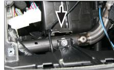
Bend down metal in order to clear space for double DIN head unit
