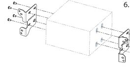
6. Attach mounting frames left/ right to double DIN head unit
