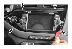
Unclip and remove OEM-panel surrounding head unit
