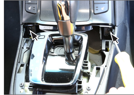
5. Remove 2 screws (see arrows)
