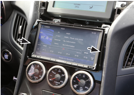
17. Put fascia plate over double DIN head unit
