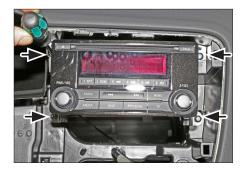
Remove 4 screws of OEM head unit (see arrows)
