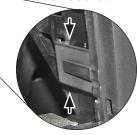
**Seat Exeo only:**The mounting frame has to be clipped behind the fixed OEM frame (see photo)
