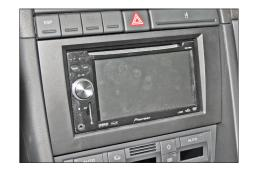
5. Connect all required circuit points and push the double DIN head unit in the metal frame until it snaps in.
