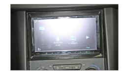
3. Put Metal Frame into dash board Connect all required circuit points
