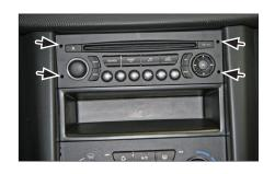
Use special radio relase keys to remove OEM head unit
