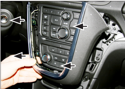
3. Pull panel towards your direction carefully
