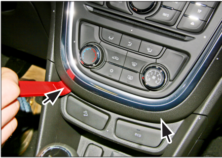
2. Unclip panel carefully (see arrows)
