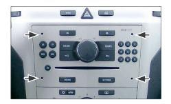
Put the radio release keys in the holes of OEM radio (see arrows)
