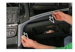
5. Unclip and remove right panel
