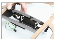
11. Clip rear side of blanking cover into OEM panel
