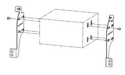
13. Mount mounting frames to double DIN head unit
