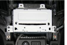
8. Remove screws of OEM head unit
